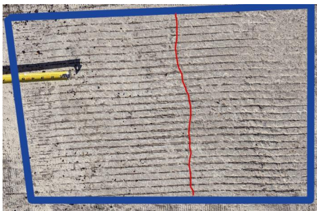
Figure B.3 Crack Formation in Patches with P4 during First (Red), Second (Green), and Third (Yellow) Inspection
