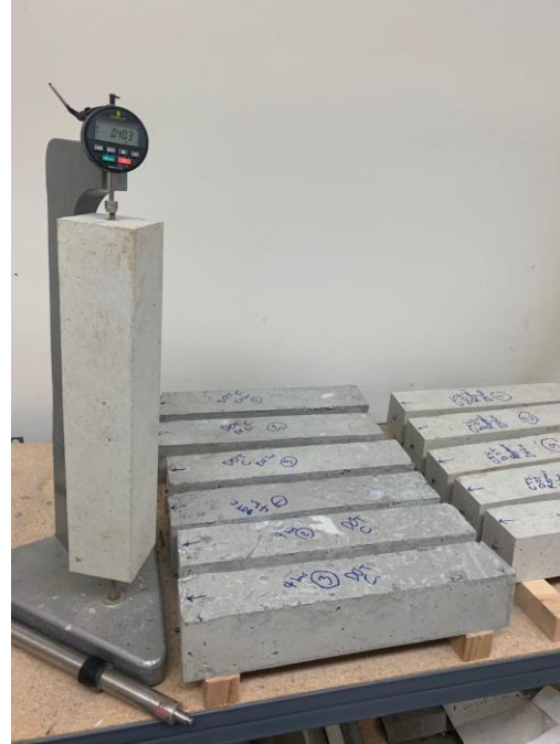
Figure 2.7 Drying Shrinkage Test Specimens and the Length Comparator
