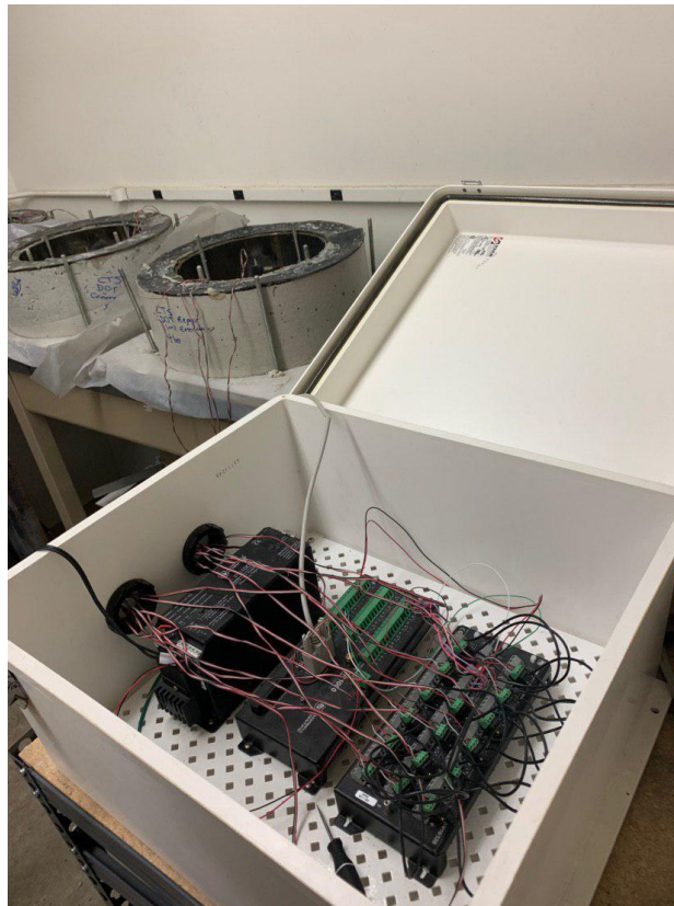
Figure 2.9 Restrained Ring Shrinkage Test Specimens Connected to the Data Acquisition System
