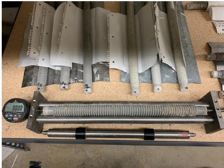
Figure 2.8 Autogenous Shrinkage Test Specimens and Measuring Device
