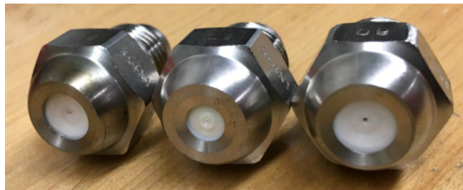
Figure 8. New nozzles being tested in the ARC-M1 combustor to evaluate ignition performance.
