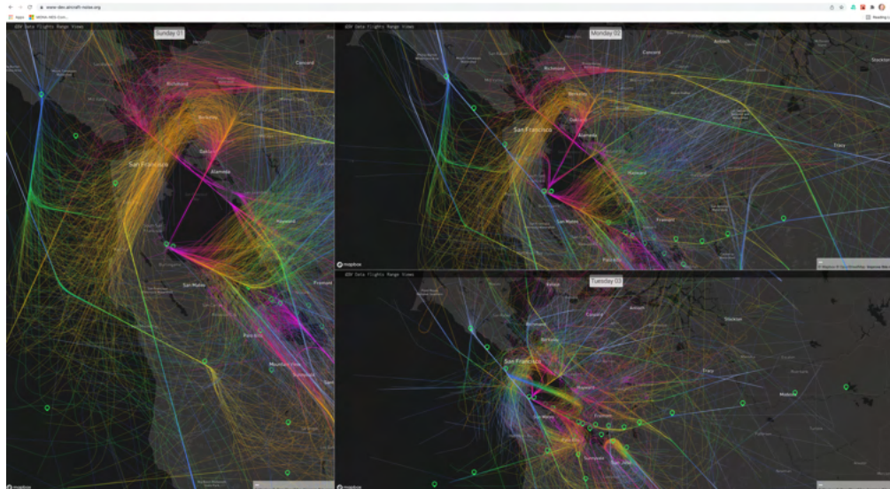
Figure 3. Comparative analysis of San Francisco Bay Area traffic patterns on different days obtained from visualization system.
