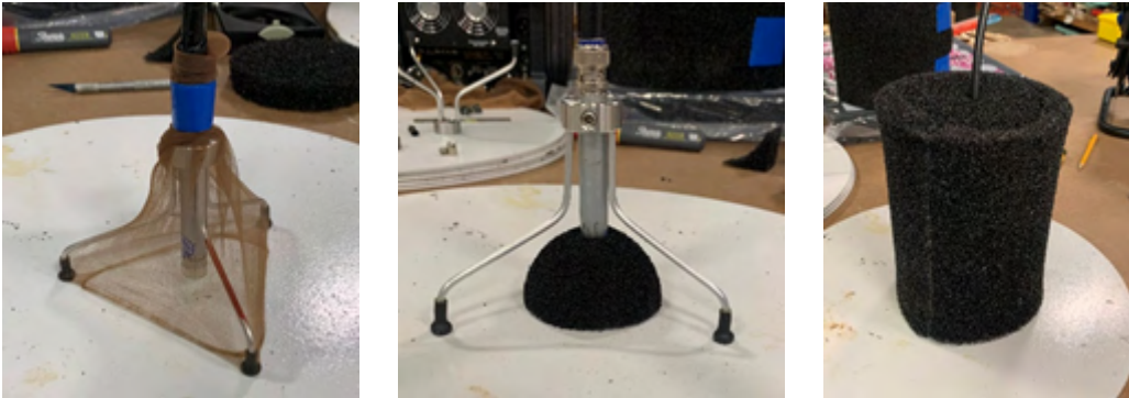
Figure 11. Nylon mesh, foam hemisphere, and foam cylinder windscreen designs.
