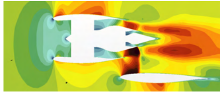
Figure 6. Mach contour plot shows the influence of the wing on exhaust streams from the engine.
