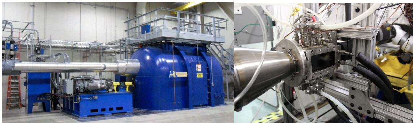
Figure 2. The SmEARF high-altitude chamber at the Army Research Laboratory at Aberdeen Proving Ground, MD (left). The M1 combustor installed in the altitude chamber, ready for cold-start and altitude relight testing (right).
