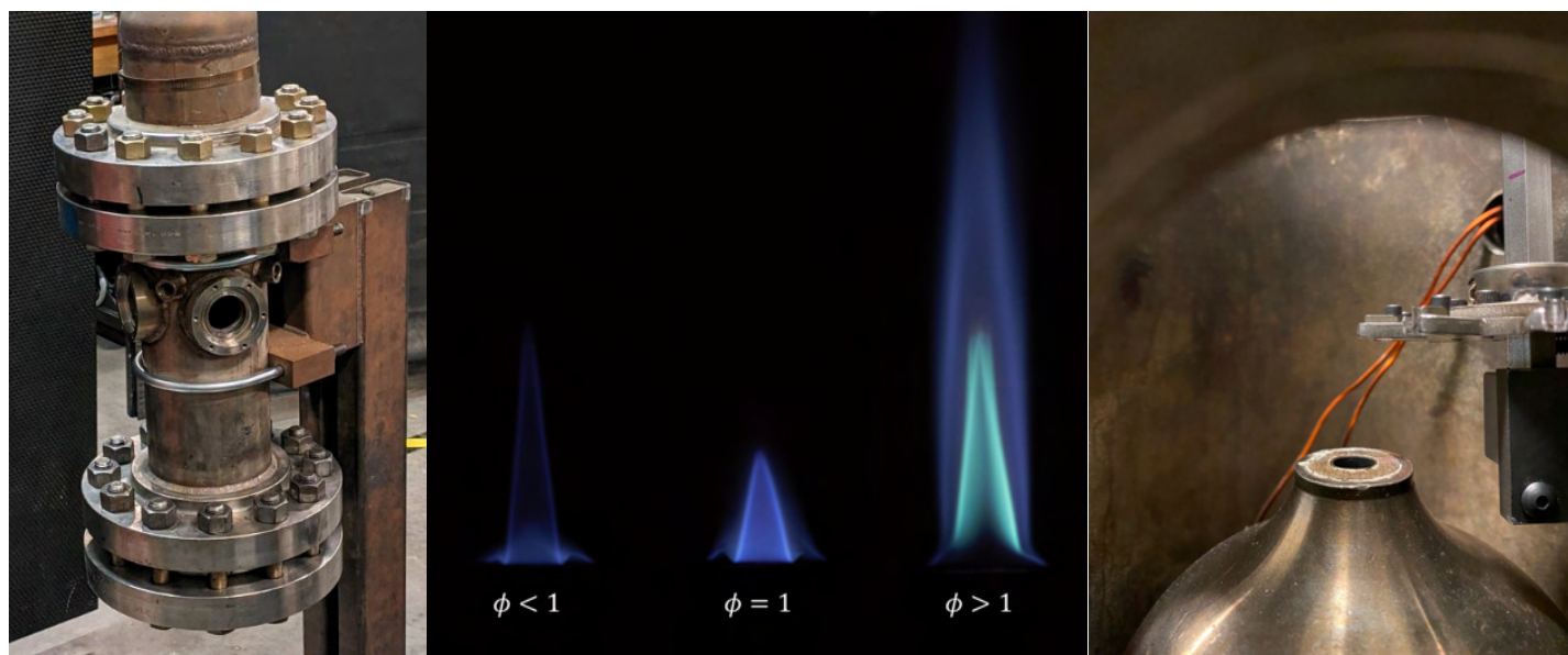
Figure 2. High-pressure calibration burner. Left: Pressure vessel. Middle: Typical laminar flames at different equivalence ratios. Right: Thermophoretic nvPM sampling system.
