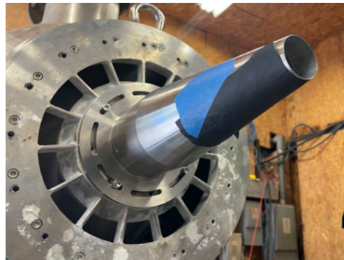
Figure 15. The 1.6-in primary nozzle installed in isolation for PIV measurement validation.
