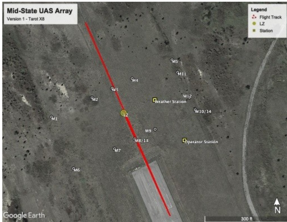
Figure 12. UAS acoustic array at Mid-State Regional Airport.
