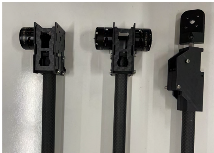
Figure 10. Three configurations for the motor mount: single, coaxial, and tiltable.
