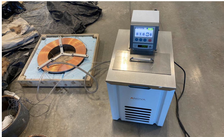
Figure 4.8 Temperature control system. Source: Tanner Research Group
