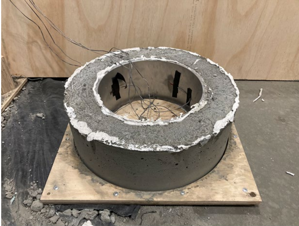
Figure 4.5 Single-ring specimen after removal of plastic cover
