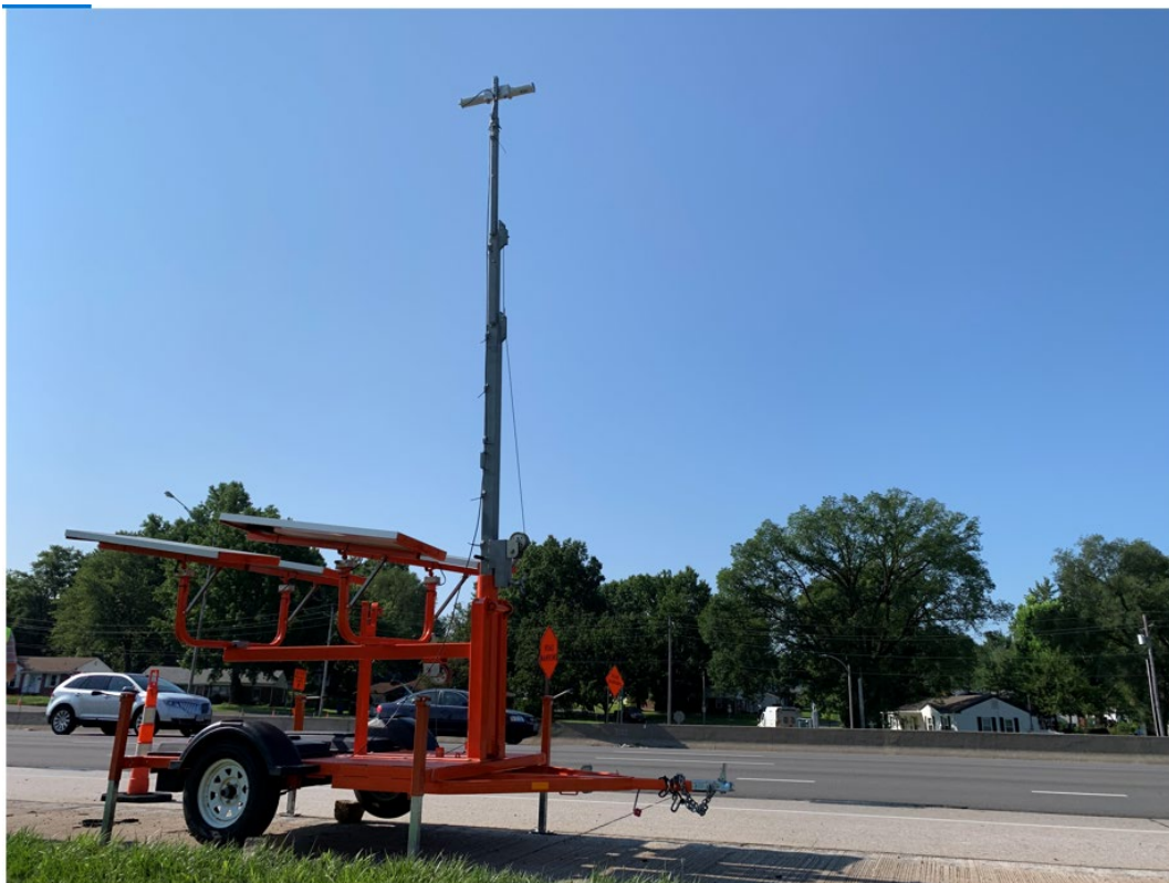
Figure 3-2. Trailer with SpeedLane® Pro sensor
