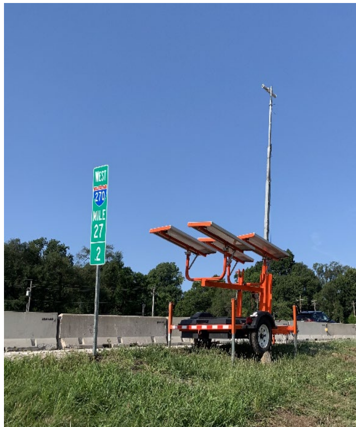
Figure 3-3. Field study upstream sensor in work zone
