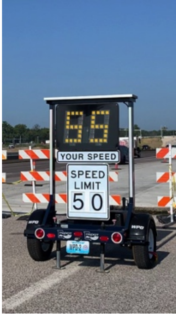
Figure 1-1. Speed display trailer deployed in work zone on I-270 near Saint Louis, Missouri
