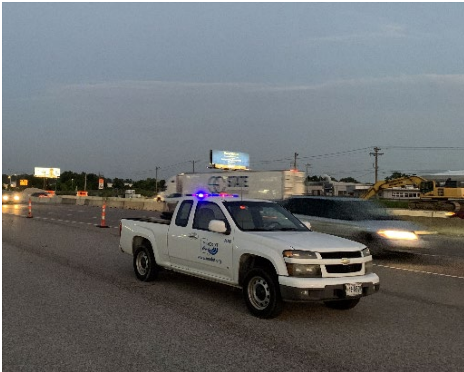
Figure 3-11. Work vehicle with red and blue lights in field study
