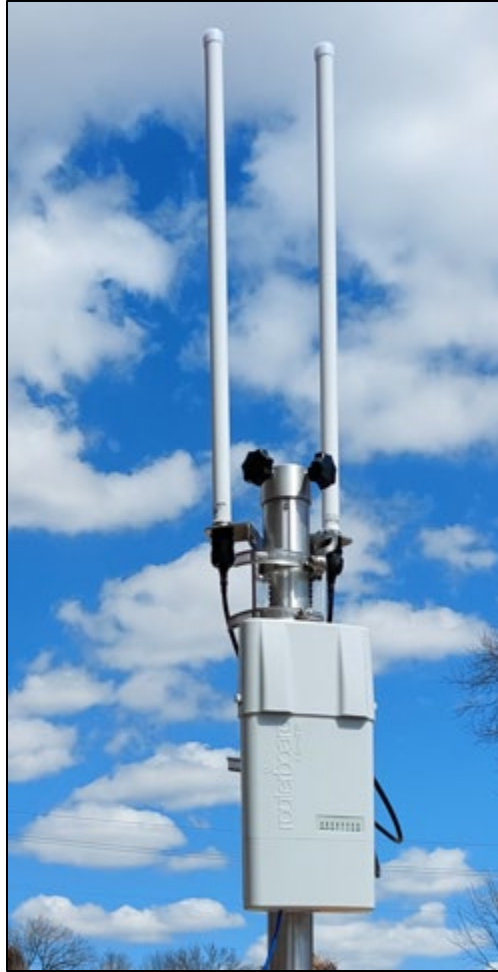
Figure 8. Photograph. An assembled Daily Use Gateway (DUG).
