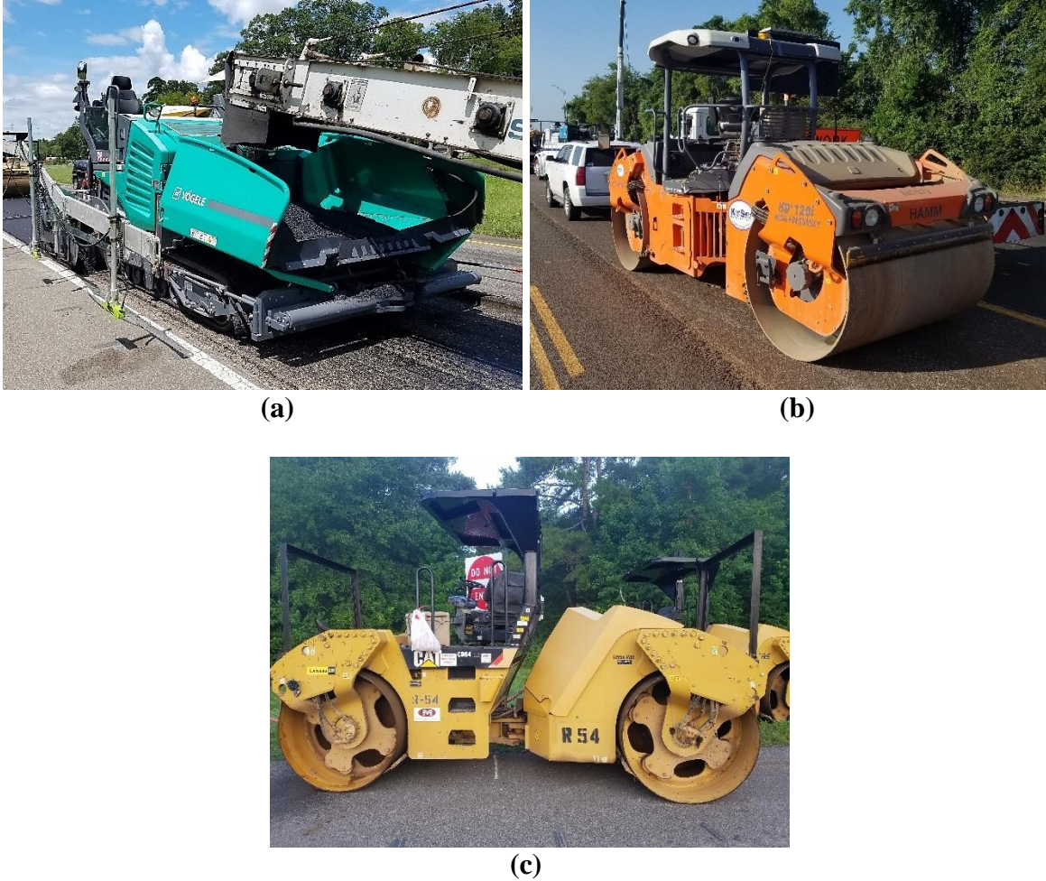
Figure 14. TYL-US 259 and ATL-US 59 Construction Equipment: (a) Tamper Bar Paver, (b) Breakdown Steel-Wheel Roller (HAMM), (c) Breakdown Steel-Wheel Roller (Caterpillar).
