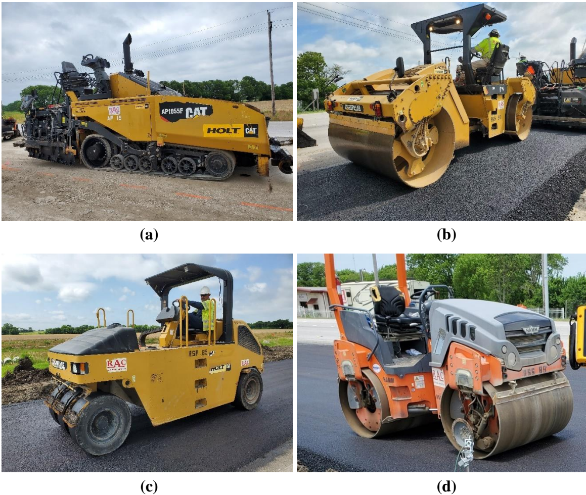
Figure 19. DAL-SH 121 Construction Equipment: (a) Tamper Bar Paver, (b) Breakdown Steel-Wheel Roller, (c) Intermediate Pneumatic Roller, (d) Finish Roller.
