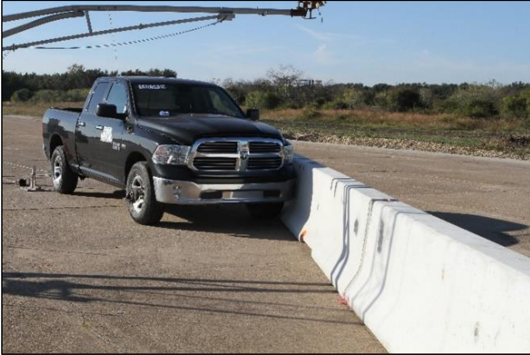
Figure 5.1. Damaged Portable Concrete Barriers/Test Vehicle Geometrics for Test No. 440592-1, Front View.
