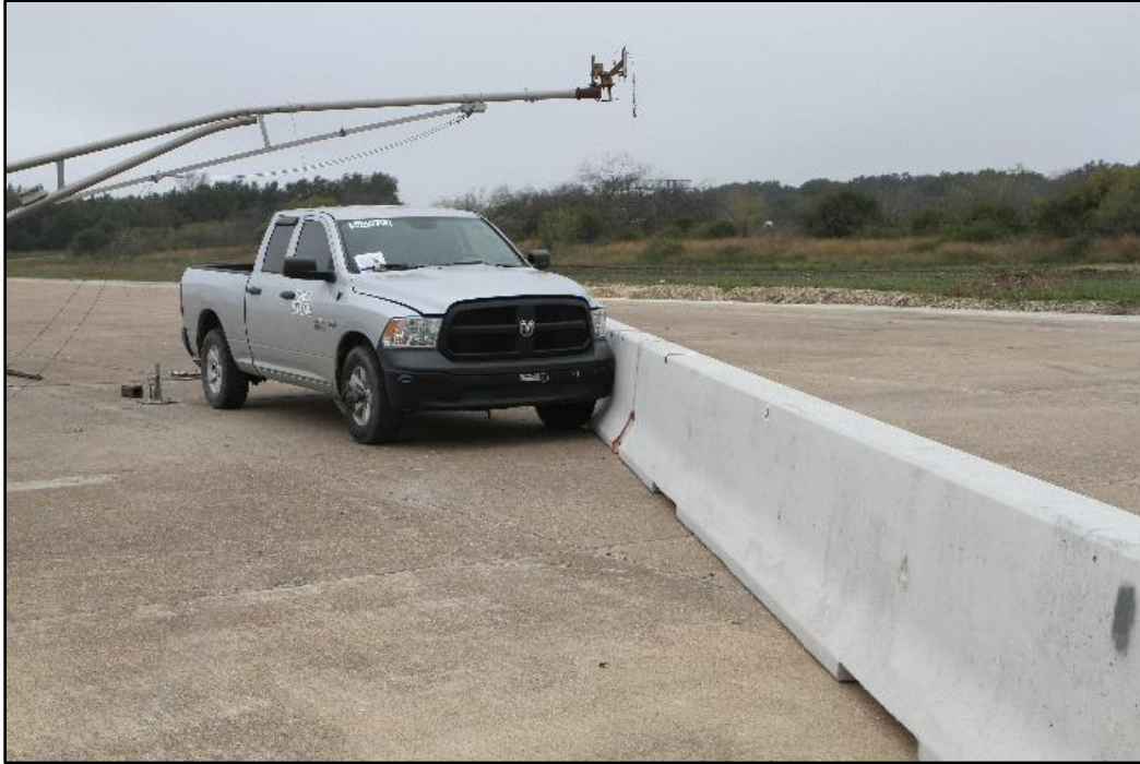
Figure 6.1. Damaged Portable Concrete Barriers/Test Vehicle Geometrics for Test No. 440592-2, Front View.
