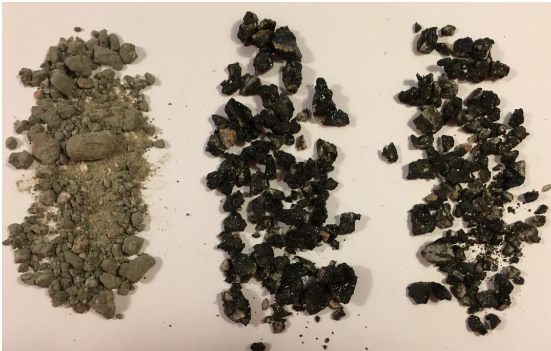
Figure 8.9. Dislodged aggregate particles from the Cantabro abrasion test method, planetary motion test method, and circular motion test method (left to right).
