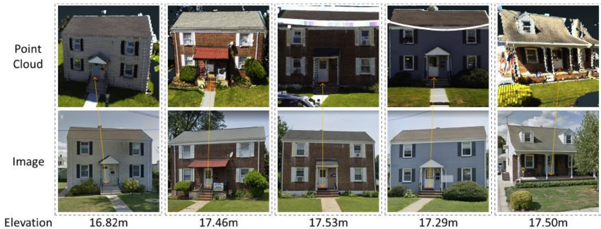
Figure 6 Examples of extraction of lowest floor elevation
