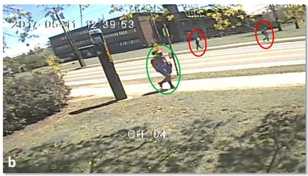
Figure 36. a) Bicyclist passes the infrared counter on a bike lane in the traveled way. b) Pedestrians on the opposing sidewalk are missed by the placement of the EcoCounter
