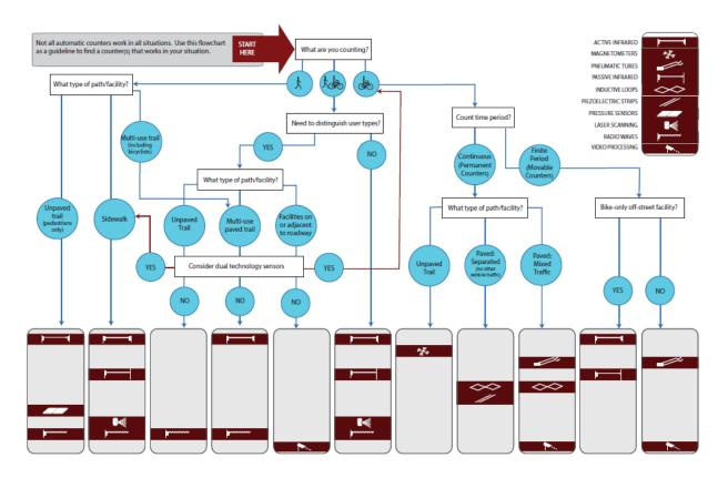
Figure 1. Data collection technology decision flowchart (Kittelson & Associates, Inc. et al., 2013).
