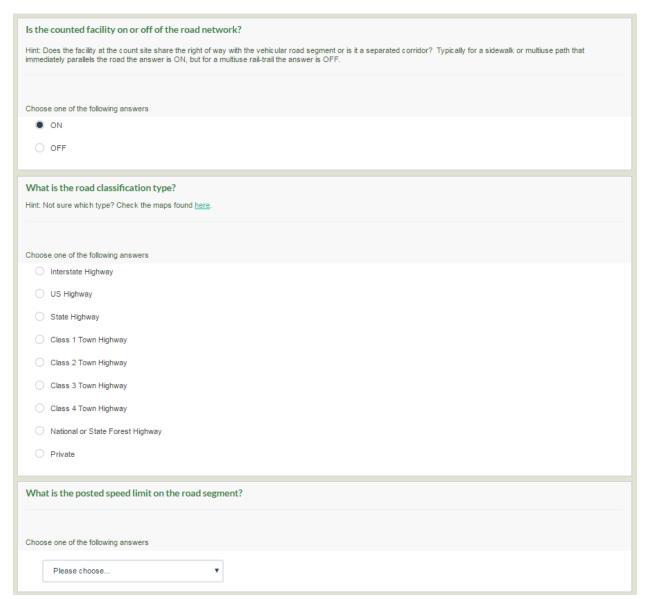
Figure 19. Defining the count facility as on-network will prompt the user to identify the road classification type and the posted speed limit.
