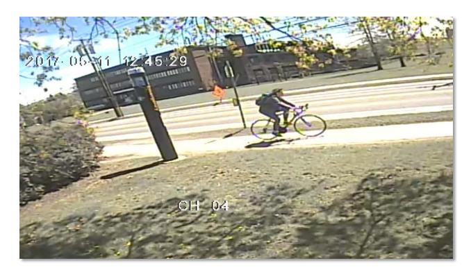
Figure 38. Example of a cyclist on the sidewalk being tallied by an infrared EcoCounter, instead of the adjacent on-road bike lane.
