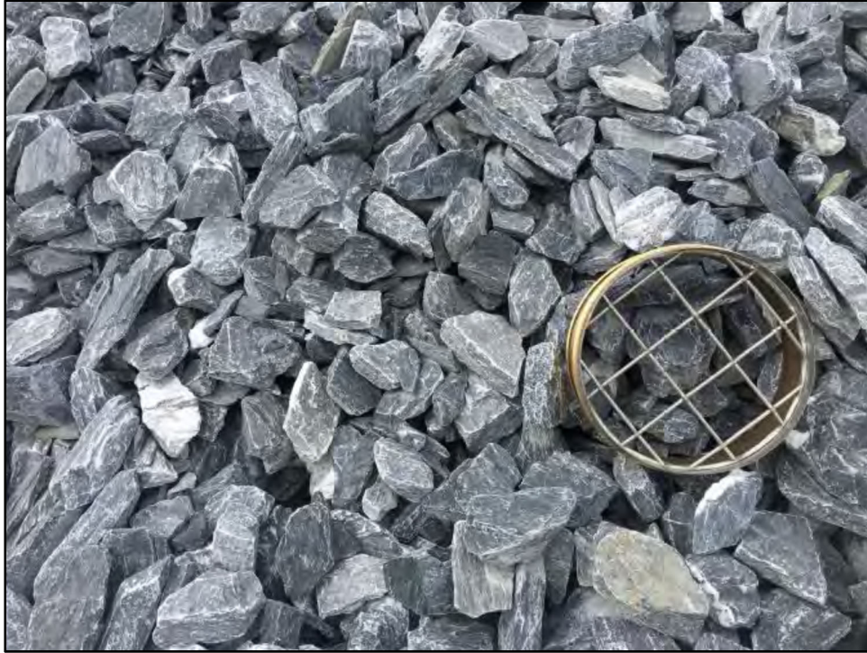
Figure 6: Stockpile of Class I ACE with a 12-inch-Diameter, 3-inch Sieve for Scale.
