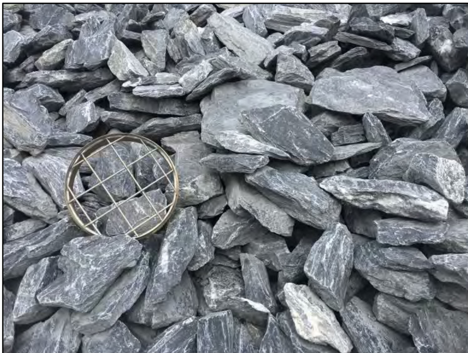
Figure 7: Stockpile of Class II ACE with a 12-inch-Diameter, 3-inch Sieve for Scale.
