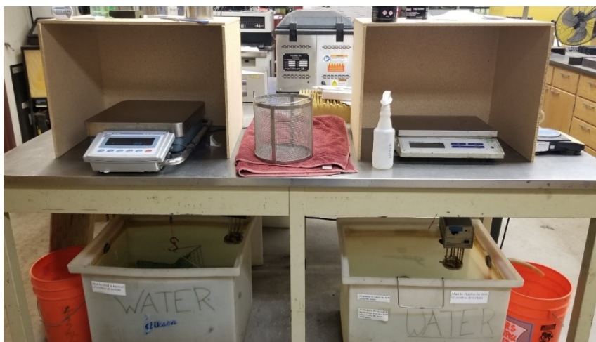
Figure 34. Coarse aggregate specific gravity and absorption testing equipment.
