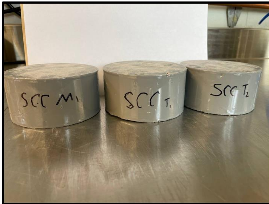
Figure 4: Cut and epoxy coated specimens before testing
