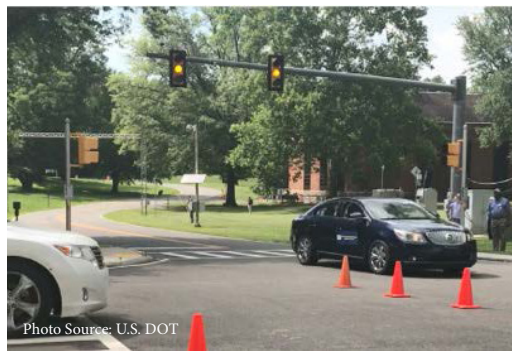
Photo Source: U.S. DOT A Tampa vehicle receives an intersection movement assist warning being triggered by a New York City vehicle
