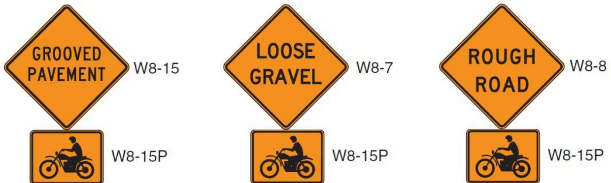
**Figure 11. Illustration. Motorcycle warning signs. Source: MUTCD, modified from source.**
