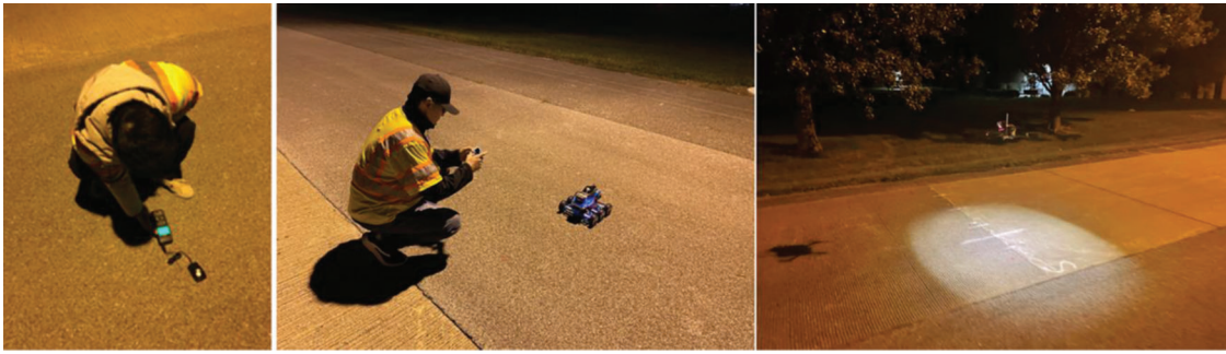
Figure 3.10 Manual (left), cart (middle), and drone (right) illuminance measurements.
