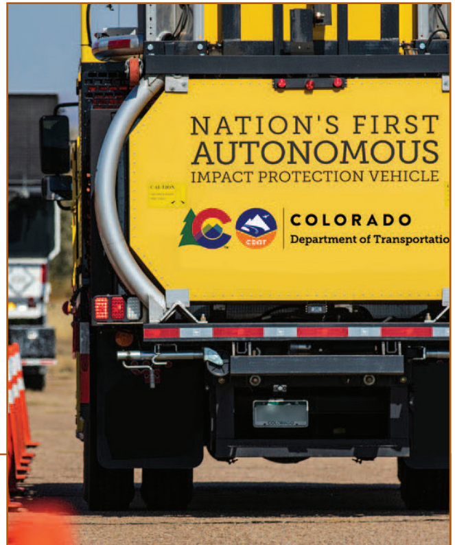
© Colorado Department of Transportation. The Colorado DOT is testing an autonomous-truck-mounted attenuator in live work zones to evaluate the safety benefits of autonomous impact protection vehicles in road maintenance.
