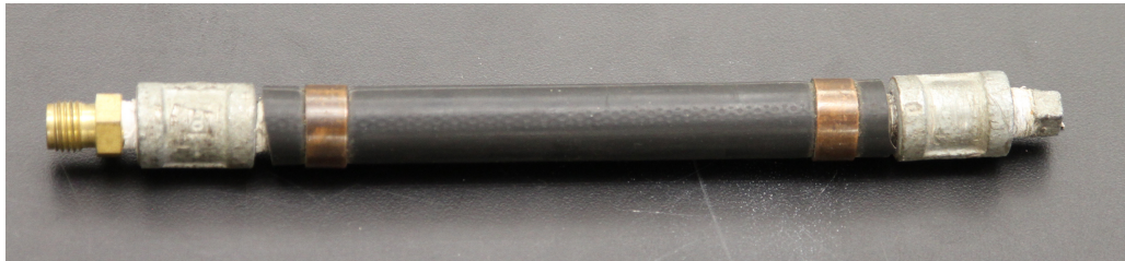
Figure 4.2: 1/8 inch Diameter Galvanized Pipe with Copper Crimp Ring Covered with Rubber Membrane, Testing Dimensions: 4.3 inch x 0.625 inch (Misilo III, 2018)
