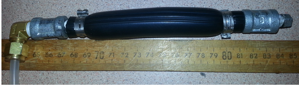
Figure 4.1: 1/8 inch Galvanized Pipe with Steel PEX Crimp Ring, partially inflated, Testing Dimensions: 4.4 inch x 0.625 inch (Misilo III, 2018)
