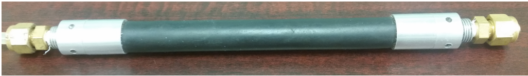
Figure 4.7: Fully Assembled Prototype SDPMT-6 Aluminum Probe, Testing Dimensions: 5.5 inch x 0.625 inch (137 mm x 15 mm) (Misilo III, 2018)
