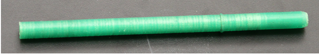
Figure 4.3: 3D Printed PLA Probe 3/8 Diameter (Misilo III, 2018)
