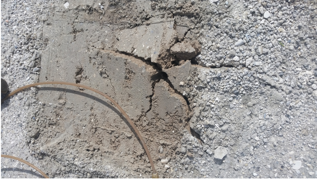
Figure 5.16: Observed Surface Cracks in Dry Cemented Coquina, 3/4 inch hole
