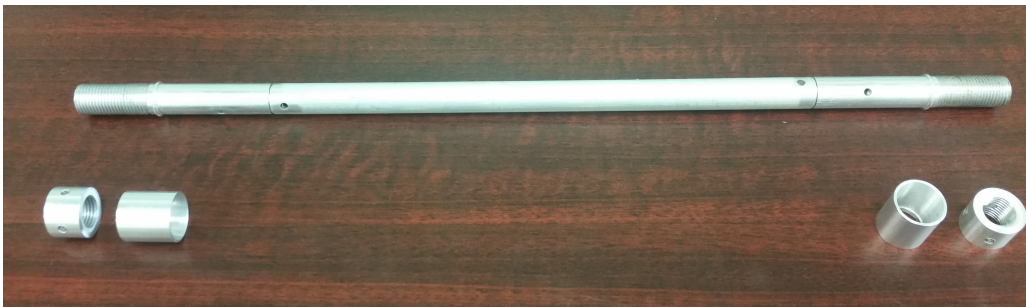
Figure 4.8: Partially Assembled Prototype SDPMT-12 Aluminum Probe Testing Dimensions: 11.5 inch x 0.625 inch (287 mm x 15 mm), probe ends (2 each), Probe Center, Nuts (2 each), and Sleeves (2 each) (Misilo III, 2018)
