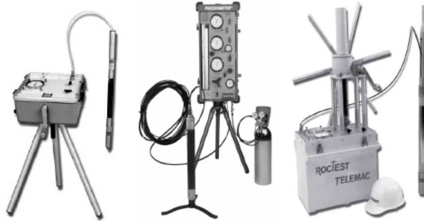
Figure 2.1: Pressuremeter Models: PPMT, Ménard PMT, and TEXAM PMT
