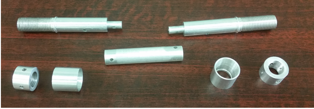
Figure 4.6: Unassembled Prototype SDPMT-6 Aluminum Probe, Testing Dimensions: 5.5 inch x 0.625 inch (137 mm x 15 mm), probe ends (2 each), Probe Center, Nuts (2 each), and Sleeves (2 each) (Misilo III, 2018)
