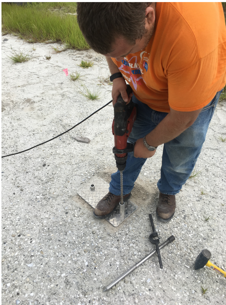
Figure 5.15: Drilling 5/8 Diameter Hole for SDPMT Testing
