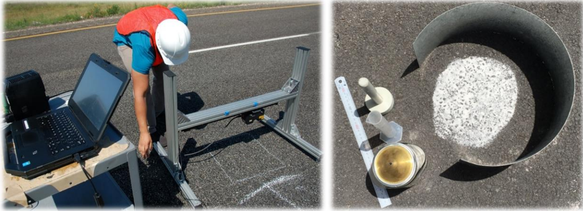
Figure 4.1 3D Laser scanner and sand patch test
