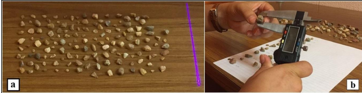
Figure A.3 a) 100 particles spread in the developed LLS prototype scanning area, and b) making measurement using a caliper
