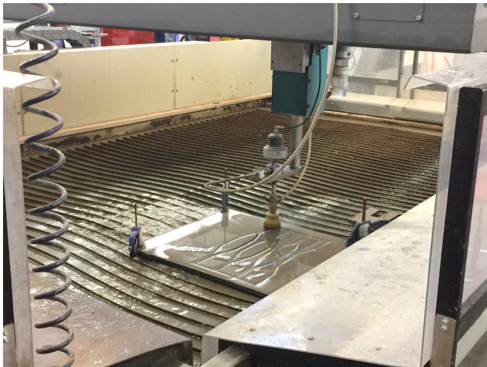
Figure 35. Fatigue sample water-jet cutting
