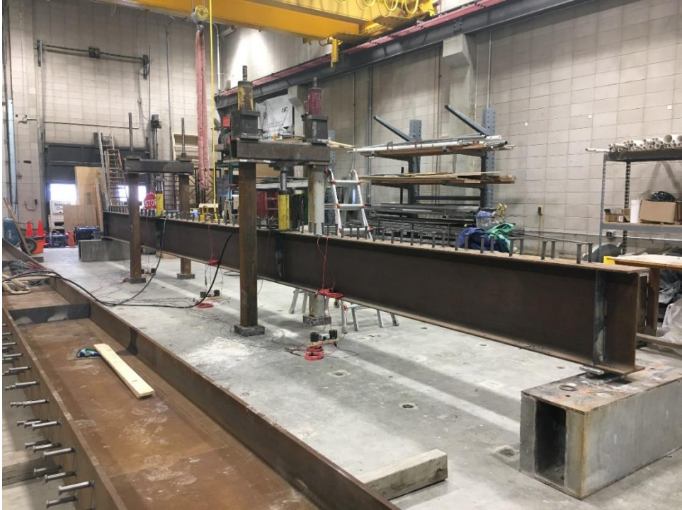
Figure 9. W24×68 non-composite load test
