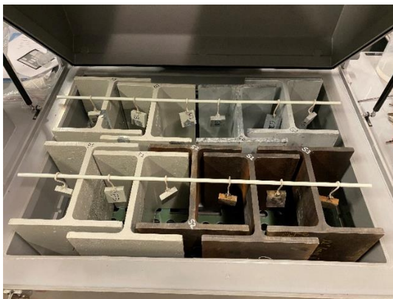
Figure 4. Samples inside the cyclic corrosion chamber
