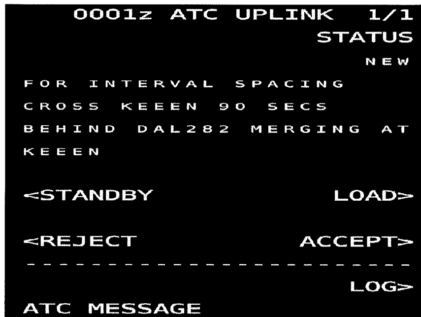
Figure 3-10. Multifunction Control and Display Unit (MCDU) Displaying Uplinked IM Clearance
