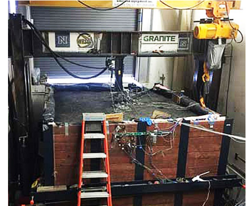
The PaveBox allows full-scale testing of asphalt pavement constructions.
