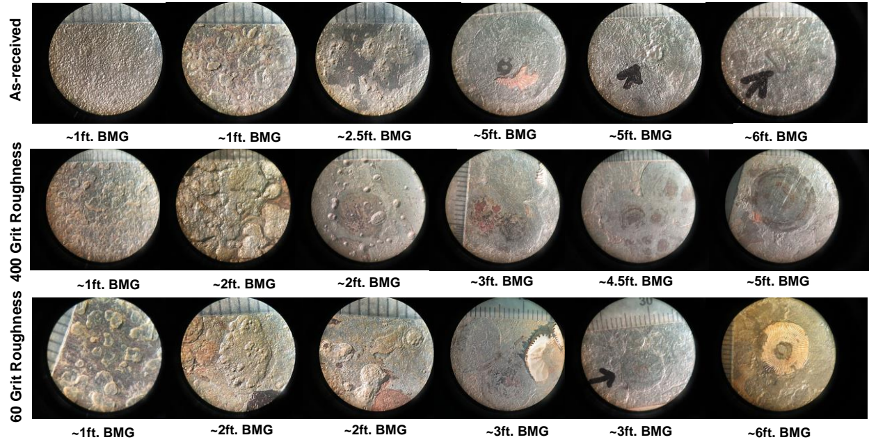
Figure 4.12. Magnified View of Surfaces of Samples from US-301 Site. Arrows highlight notable features such as pitting, surface corrosion, remnant barnacle location. Rule at 1 mm intervals.
