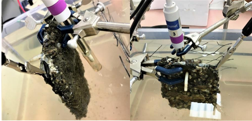
Figure 6.2. Example of Laboratory Electrochemical Test Setup.
