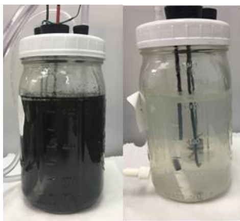
Figure 5.5. Visual Indication of Iron Sulfide Precipitation in Test Solution. Left- Inoculation with SRB. Right- control case
