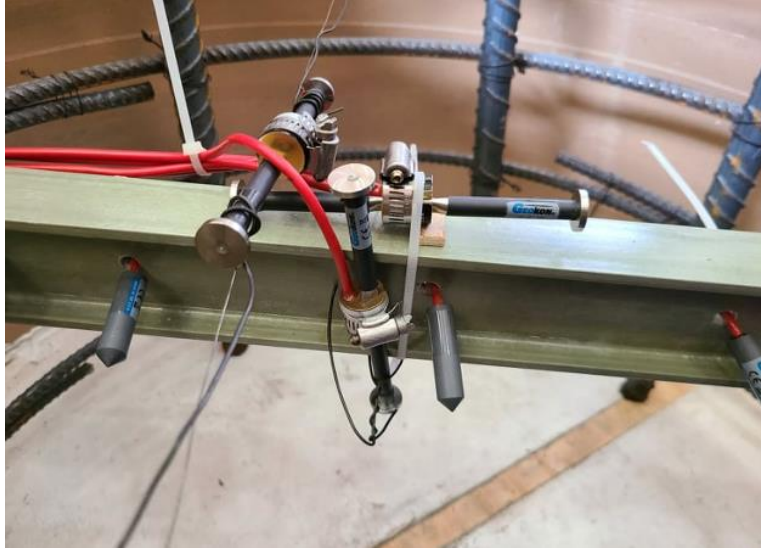
Figure 13. Photo. Vibrating wire strain gauge sensor configuration at the center of the air specimen
