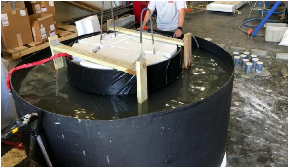
Figure 25. Photo. Test C-W-A specimen after casting and filling the tank with water
