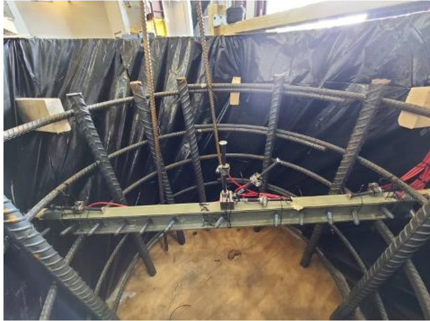
Figure 15. Photo. Sensor configuration used in both the water and soil samples
