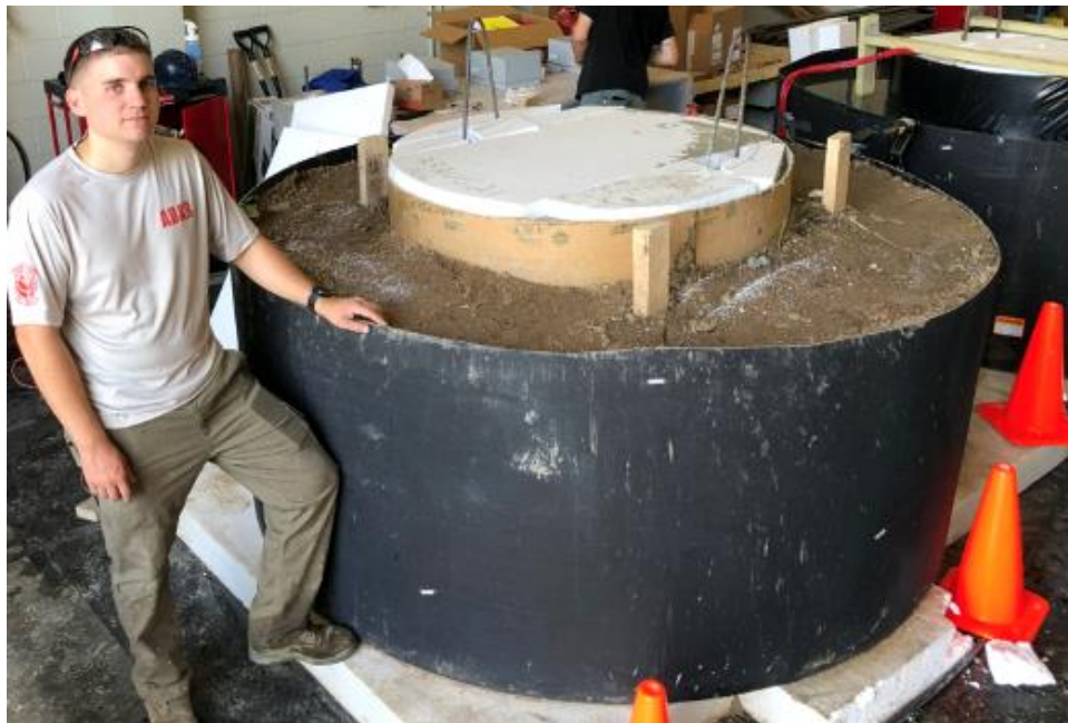
Figure 22. Photo. Test C-S-A specimen after soil placement
