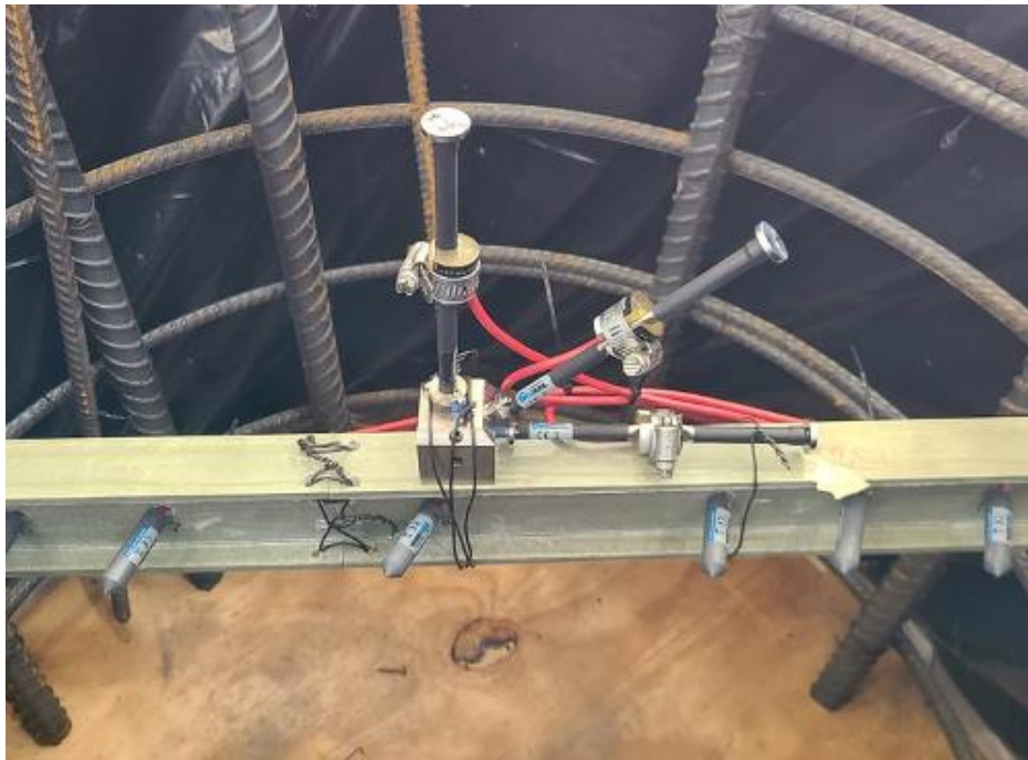
Figure 14. Photo. Strain rosette configuration used in the center of the water and soil specimens
