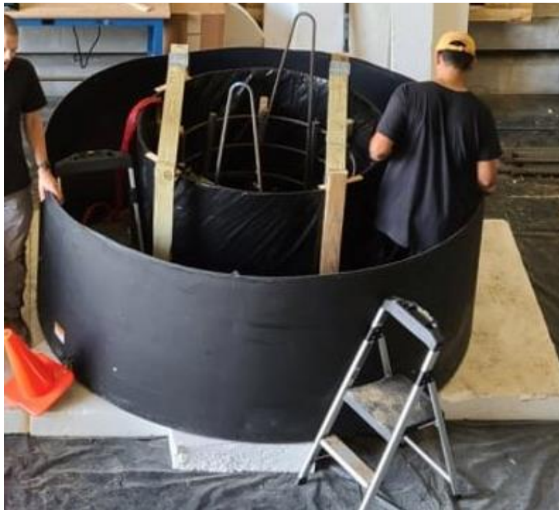
Figure 24. Photo. Water specimen experimental setup prior to concrete placement
