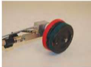
Wheel electrode with moistening wheel for continuous wetting up to a length of 200m (650ft). Linear distance recorder with travel direction detection. Automatic measurement at pre-selected intervals.
