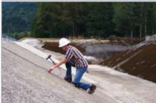
Determine areas of void/poor subgrade support and flawed concrete conditions with Slab Impulse Response
