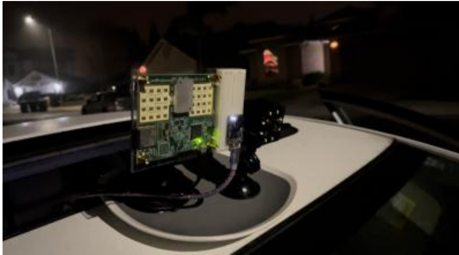
Figure 25. Live Demonstration of Pedestrian Detection at Night: System Setup on a Vehicle
