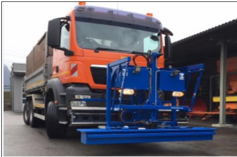
Figure 2.9: Truck mounted with rumble strip pick and place machine (Trafficsafetysystems.eu, n.d.)
