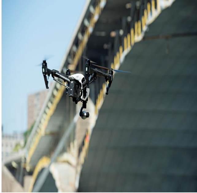
Figure 34 Bridge Manual Inspection Using Drone (Source: www.roadbridges.com )
