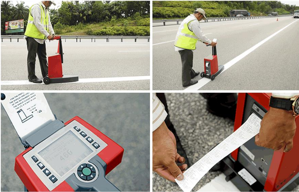
Figure 37 Pavement marking retro-reflectometer (Source: Kemakmuran Group)
