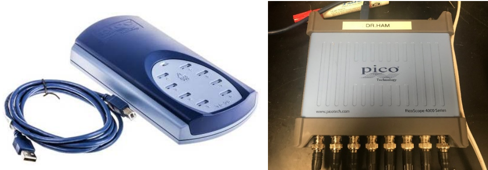
Figure 5. DAQ system: PicoScope TC-08 USB for acquisition of the thermocouples signals (left), PicoScope 4842 for acquisition of the accelerometers and the MEMS sensor's signals (right)
