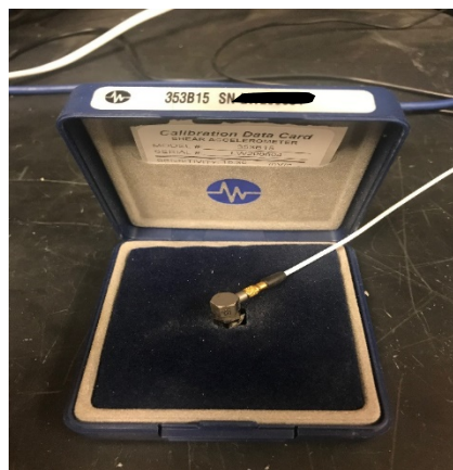
Figure 6. Piezoelectric sensor for vibration measurement
