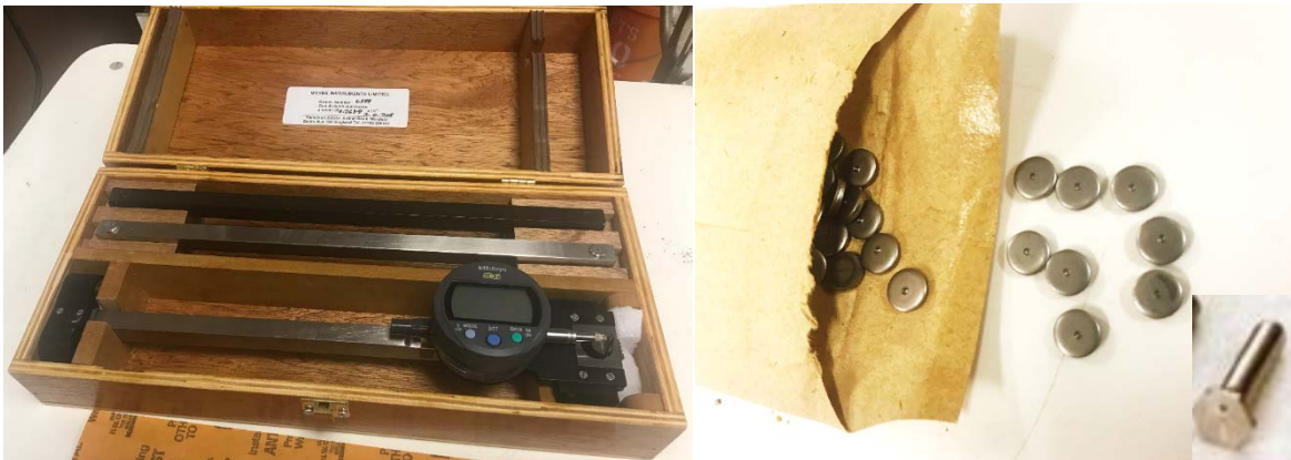
Figure 4. The Demountable Mechanical Strain Gauge (DEMEC): 300 mm DEMEC (left), 1mm drilled stainless steel disks and bolt (right).
