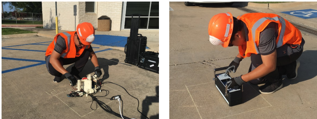
Figure 59. RACM (left) and MIRA (right) test on the parking lot site
