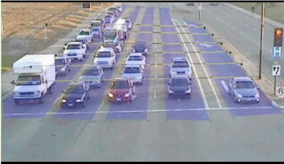
Figure 2.2 InSync cameras detection through image processing [6]
