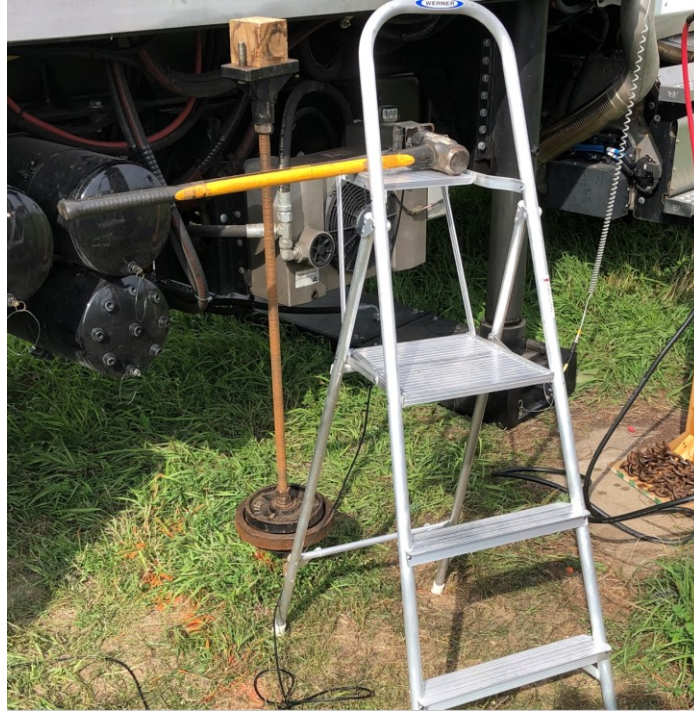
Figure 2.6 Hammer impact method configuration.
