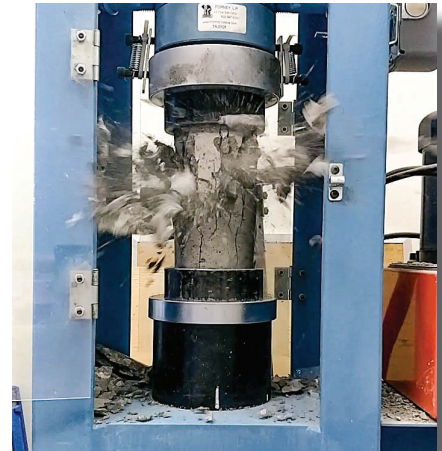
ASTM C39 compressive strength testing of concrete specimen
