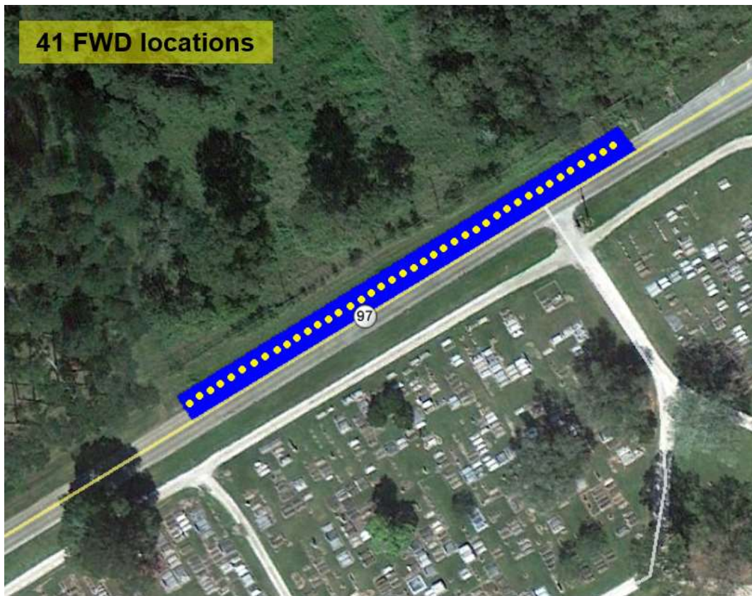
Figure C6 FWD test locations along LA 97
