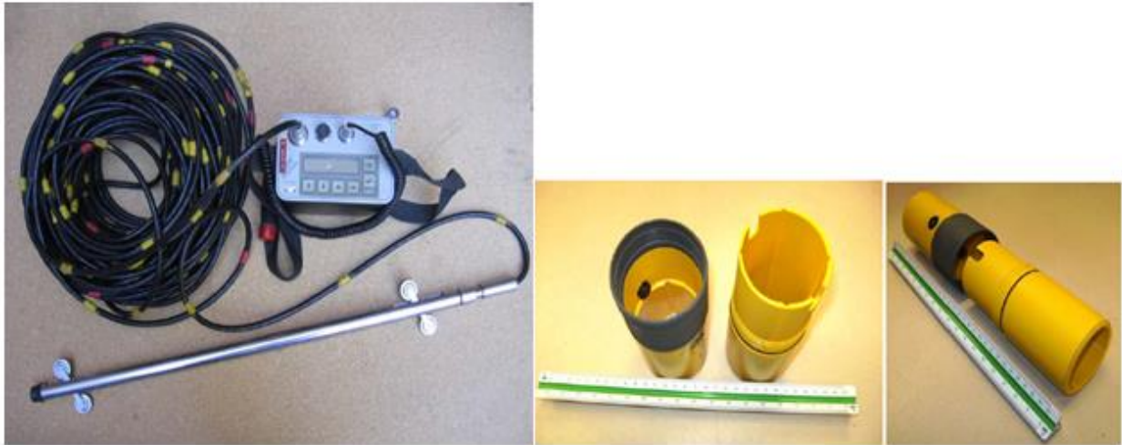
Figure 18. Typical slope inclinometer parts and inclinometer casing
