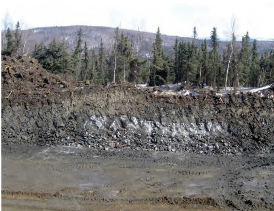
Figure 8. Wedge ice exposed on the right side at station 477+00. Tracing the wedge in the floor of the cut revealed with wedge was cut at an oblique angle.
