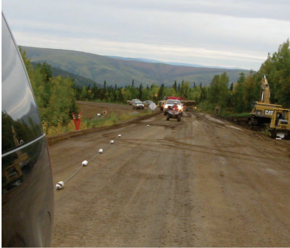
Figure 3. Photo taken during the survey with five receivers in the foreground and behind the black towing vehicle, and the transmitter in the background with the ATV guide at the very end of the system.
