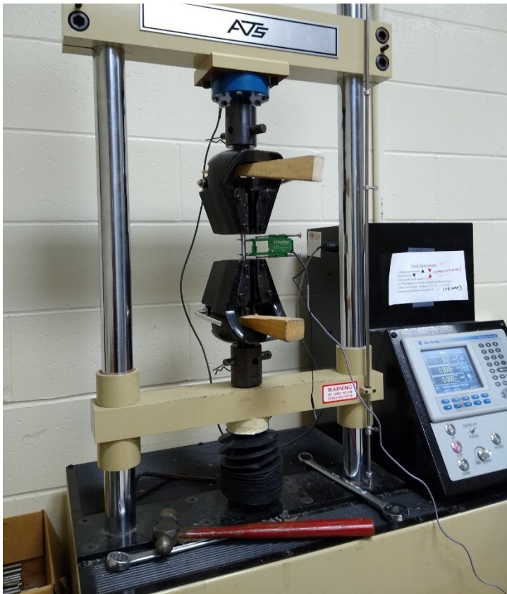
Figure B.14: Steel reinforcement during tensile test.
