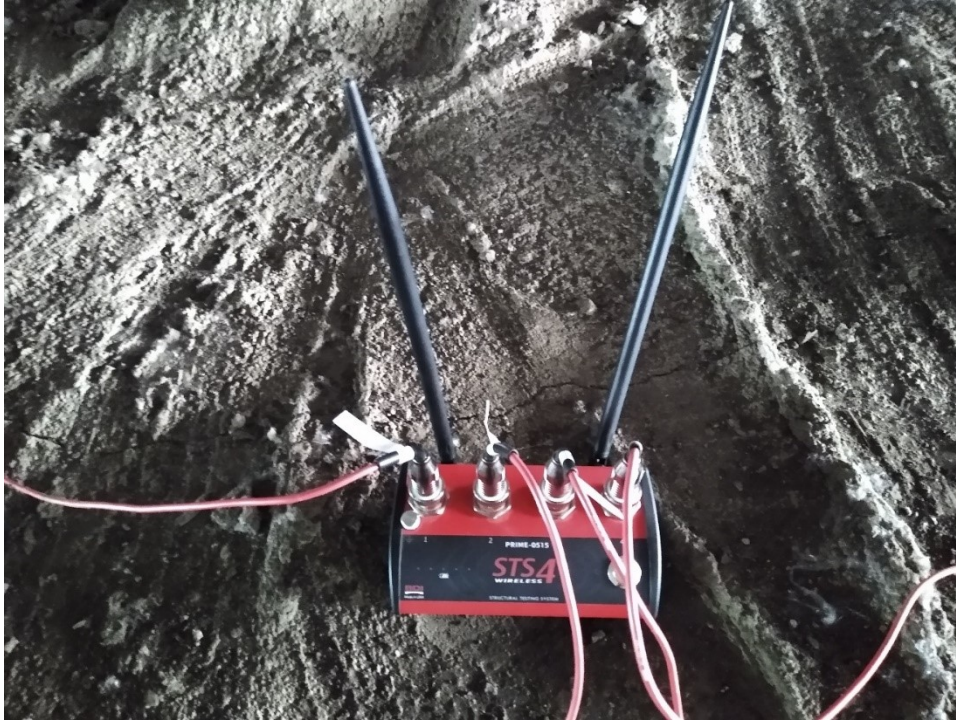
Figure F.3: Bridge Diagnostics four-channel node used for data collection.
