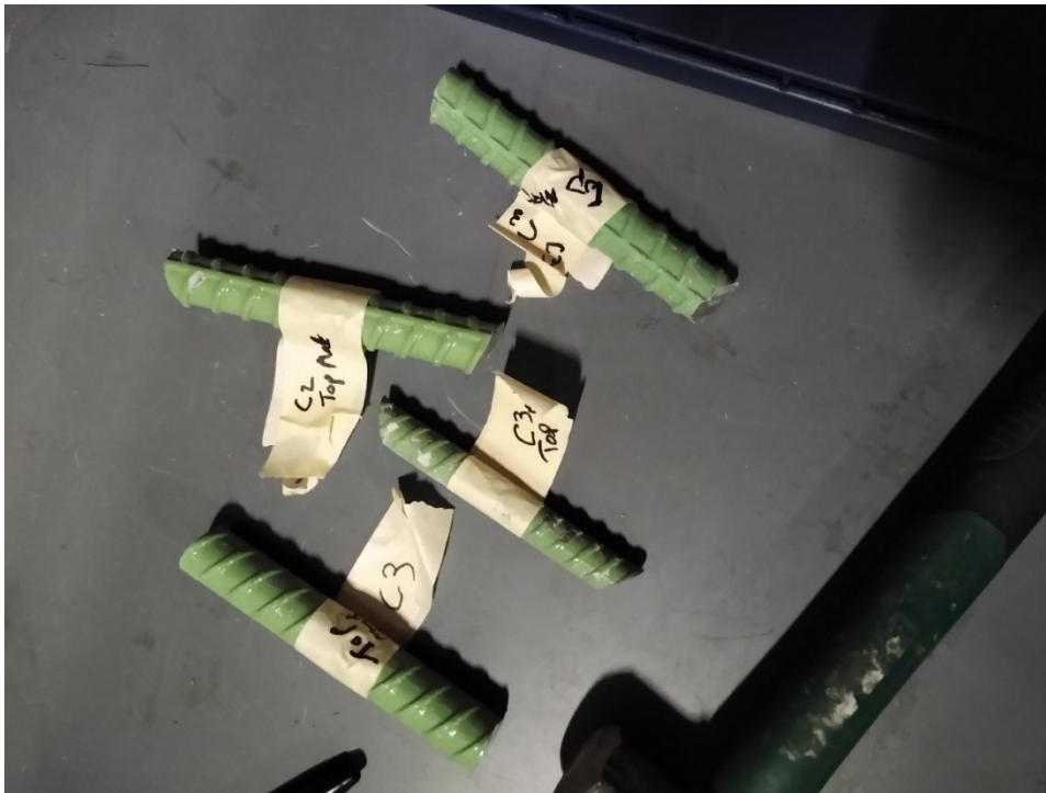
Figure B.12: Epoxy coated steel reinforcement obtained from 6 in. cores from Bridge 27926.
