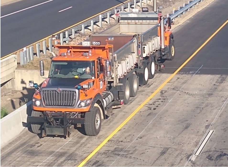
Figure H.7: Back-to-back trucks at the West span of Bridge 27925 (L1T1W).
