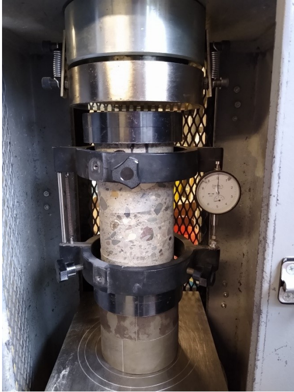
Figure B.11: 4 in. core prepped for elastic modulus test.
