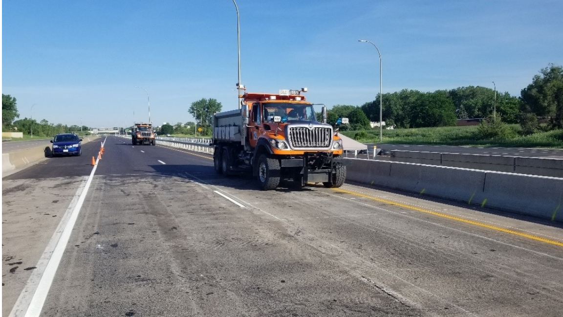
Figure 3.20: Single truck test.
