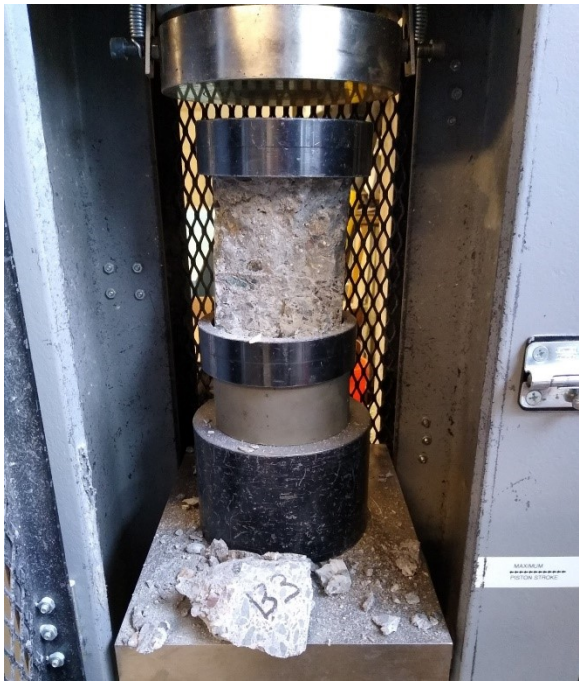
Figure B.10: 4 in. core broken in compression.
