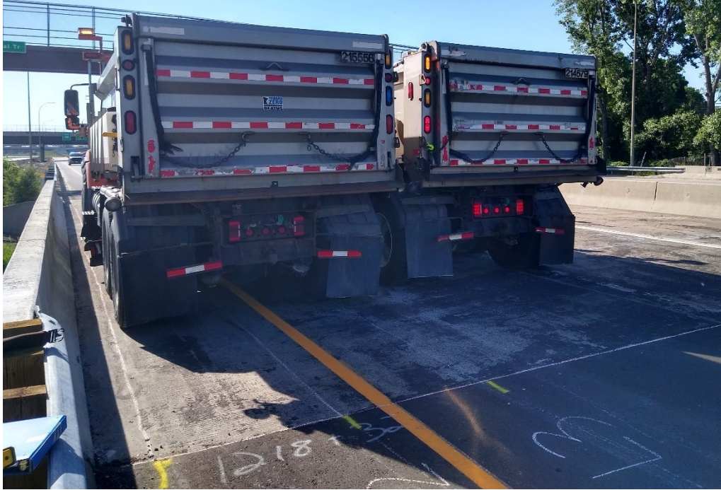
Figure F.9: Side-by-side truck test on the West span of Bridge 27926.
