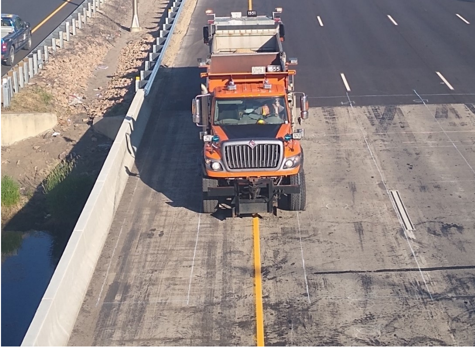
Figure H.8: Back-to-back trucks at West span of Bridge 27925 (L2T1W).
