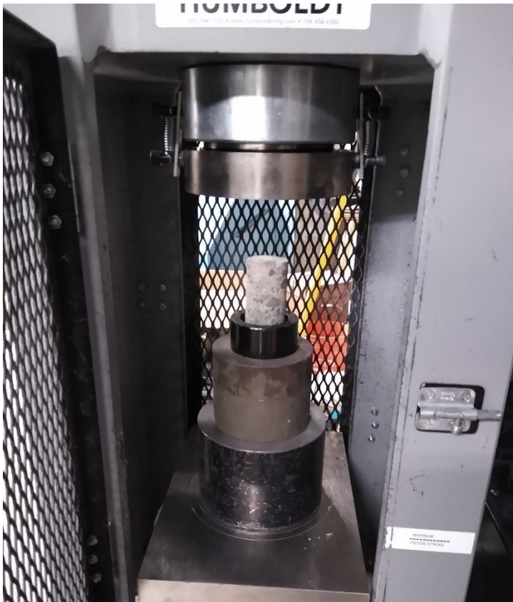
Figure B.8: 1.75 in. core prepped for compression test.
