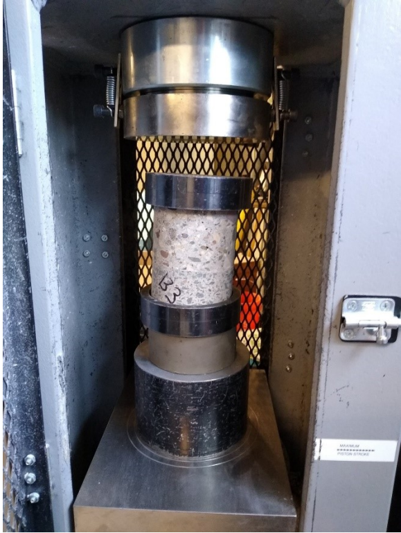
Figure B.9: 4 in. core prepped for compression test.
