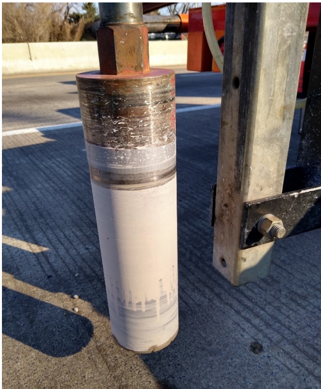
Figure B.4: 6 in. core bit.
