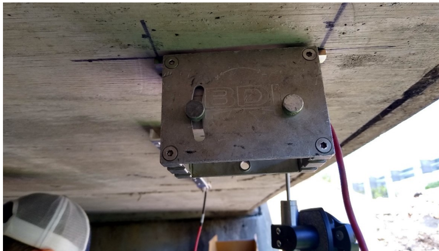
Figure 3.14: Tiltmeter affixed to the slab of Bridge 27926 during field testing.
