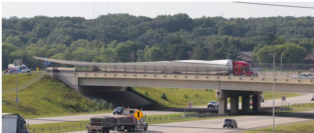
Figure 1.2 OSOW vehicle hauling a windmill blade
