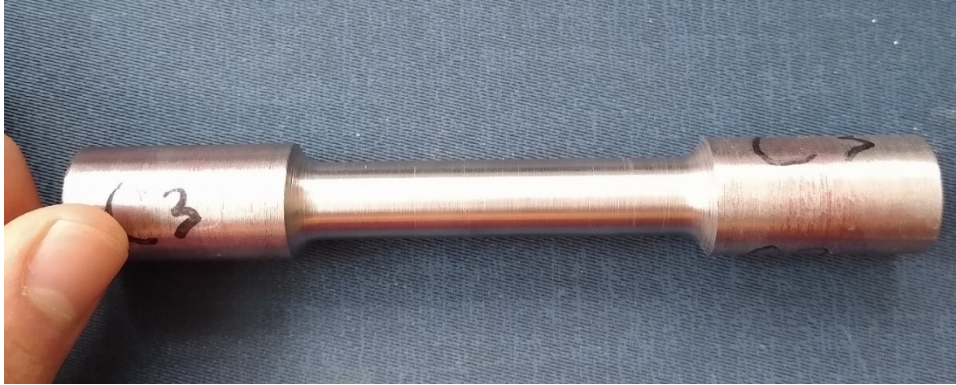
Figure B.13: Steel reinforcement machined for tensile testing.
