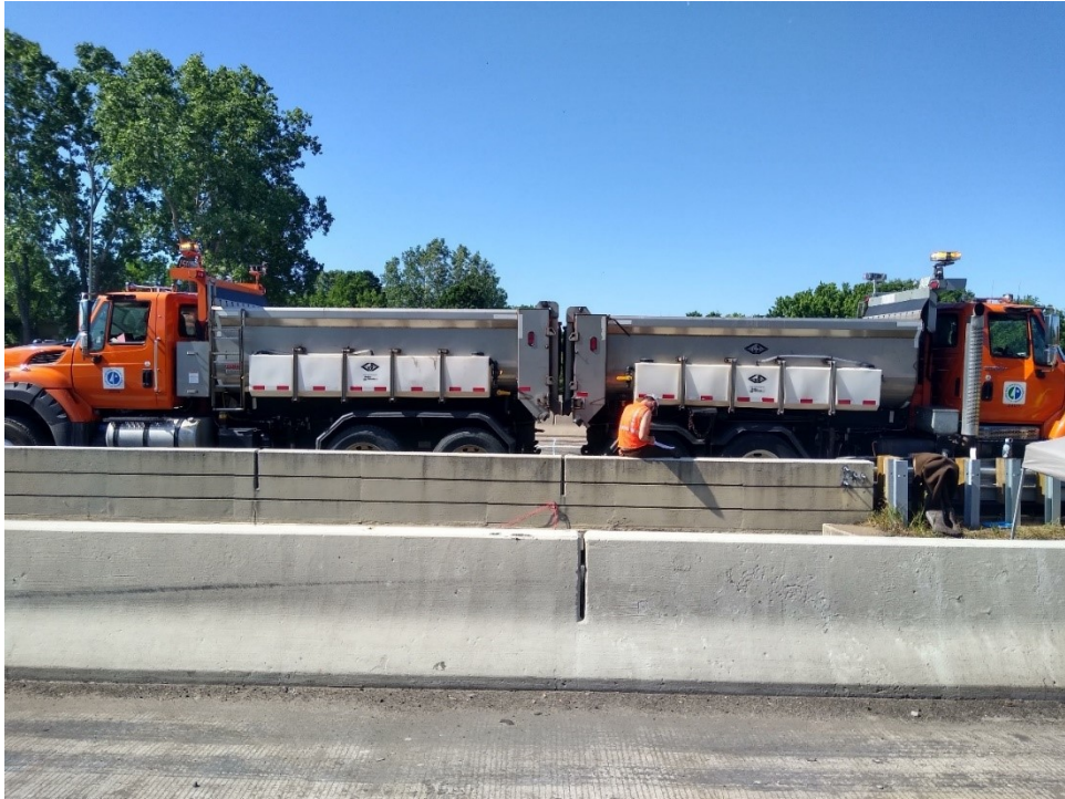
Figure F.10: Back-to-back truck tests on Bridge 27926.
