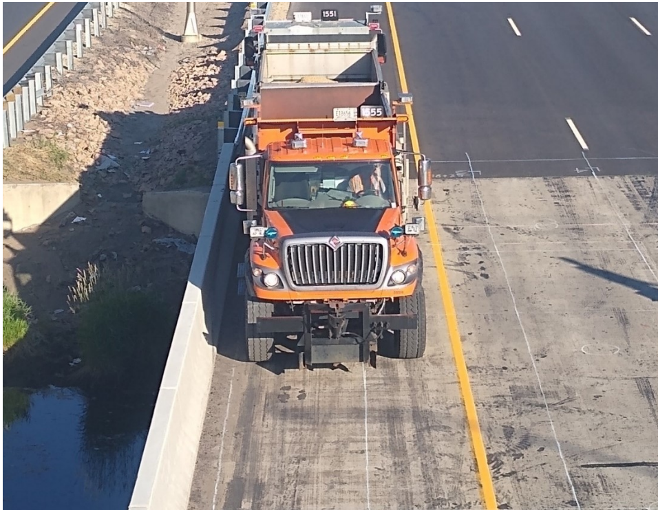
Figure H.6: Back-to-back trucks at the West span of Bridge 27925 (L1T1W).
