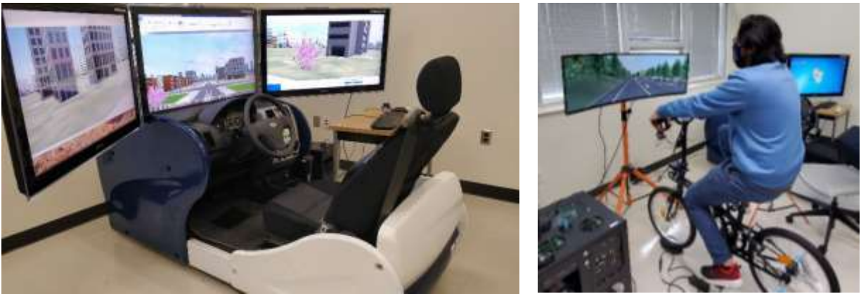
Figure 5: Car and Bike simulator
