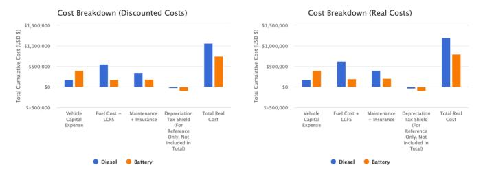
Figure 2. Cost Breakdown from Payback Analysis (Adapted from <a href="https://californiahvip.org/tco/">https://californiahvip.org/tco/</a>)
