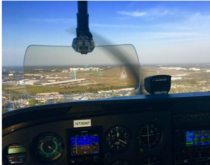
Figure 5. Research HUD on a high-wing Cessna 172
