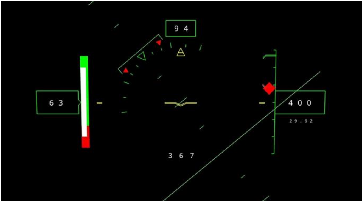
Figure A- 15. The pilot initiates a maneuver at low altitude that produces an unacceptable energy state. The airspeed will need to be increased or the bank angle returned to the acceptable envelope to return to the inside of the “energy funnel.”
