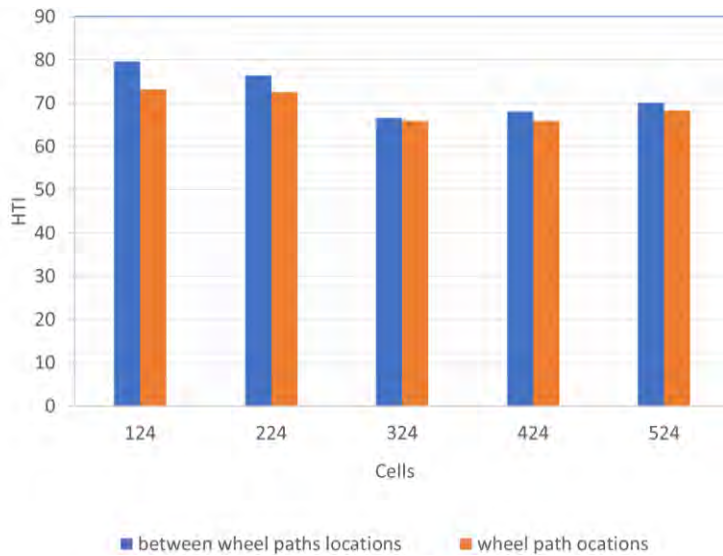
Figure 7.9 Mean HTIs at the core locations, inside lane
