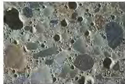
Magnification: 30x Description: Hardened air void system
