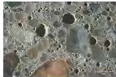
Magnification: 30x Description: Hardened air void system
