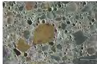
Magnification: 30x Description: Hardened air void system
