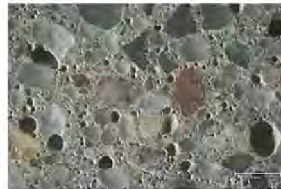
Magnification: 30x Description: Hardened air void system
