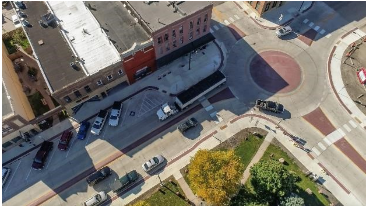
Figure 3.24 Aerial view of downtown St. James, showing mini-roundabout and back-in parking stalls
