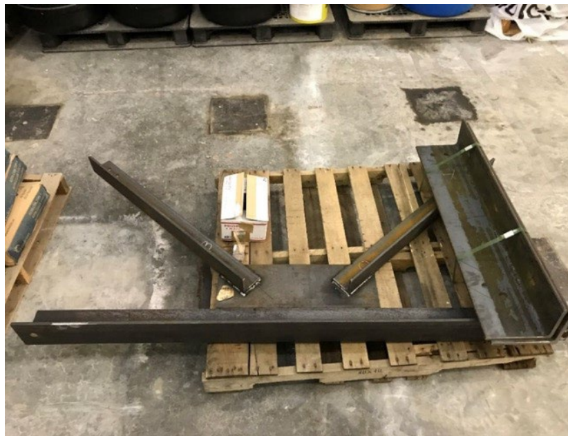
Figure 21. Photo. Fabricated k-frame replica
