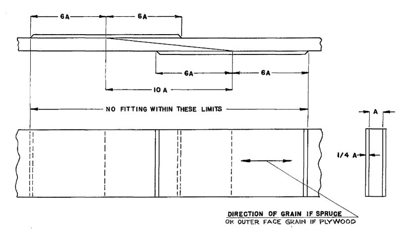
REINFORCING PLATES TO BE SPRUCE OR PLYWOOD AND SHALL BE GLUED ONLY.
