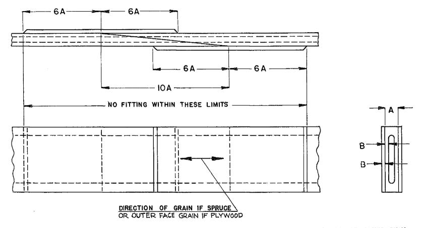
REINFORCING PLATES SHALL BE SPRUCE OR PLYWOOD AND SHALL BE GLUED ONLY.
