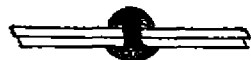
BODY OF RIVET TOO SHORT. CLOSING HEAD SHAPED TOO MUCH WITH SNAP DIE.
