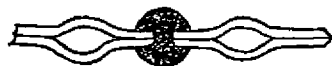
RIVETED TOO MUCH. RIVET BODY CLINCHED TOO MUCH, PLATES CLINCHED AT RIVET AND DRIVEN APART.
