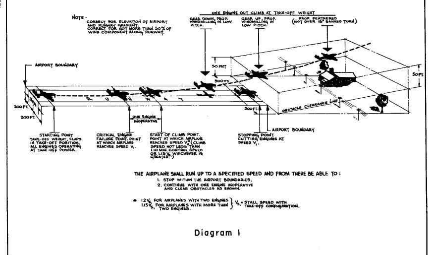
$V_2$ =climb out speed, feet per second, true air speed.
