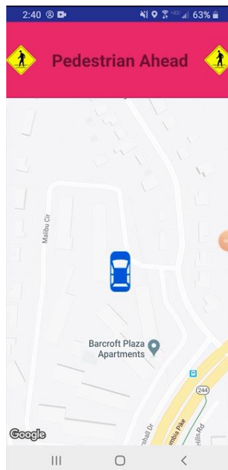
Figure 2. Screenshot. In-vehicle warning provided by the Mid-block app. The display was accompanied by alert tones and the audio message: “pedestrian ahead.”
