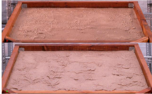
b. 24h cured 3% XG medium sand. Top: 15° Bottom: 20°
