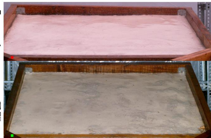
b. 24h cured 3% XG fine sand. Top: 10° Bottom: 25°
