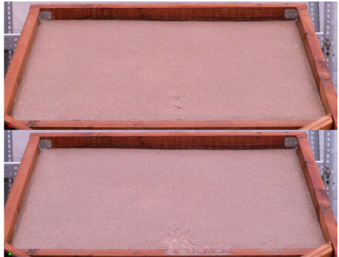
b. 24h cured 1% X.G. medium sand at 25°. Top: 15 min Bottom: 20 min
