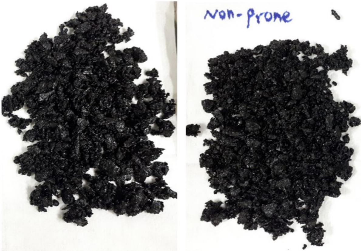
Figure 27 - Photos of HMA mixture after boiling water test (a) mixture with prone aggregate, and (b) mixture with non-prone aggregate
