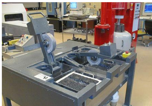
Figure 7 - Hamburg Wheel Tracking test device (source: Pavement Interactive, 2022b)
