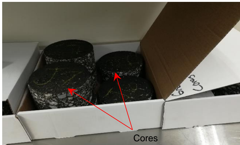
Figure 13 - Photo of the received asphalt cores in a box
