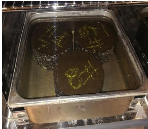
Figure 21 - Photo of the asphalt cores submerged in a water bath at 140 °F
