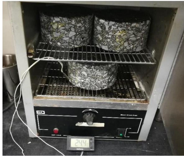
Figure 22 - Photo of dry cores inside the oven maintained at 77 °F (i.e. test temperature)
