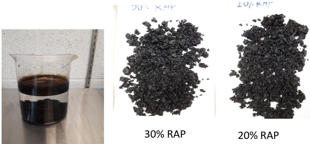
Figure 26 - Boiling water test to evaluate the effect of additional RAP in the mixture
