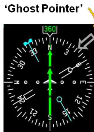
Figure 18. HSI with ‘ghost’ pointer roll out guidance when flying an RF leg
