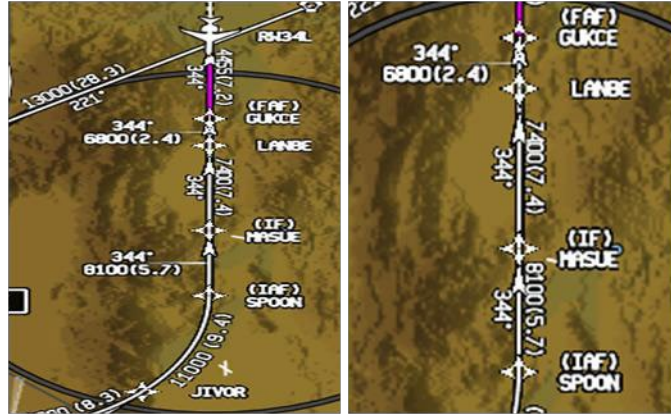
Figure C.6.1: Benefits of an offset pointer drawn to the area where the data belongs
