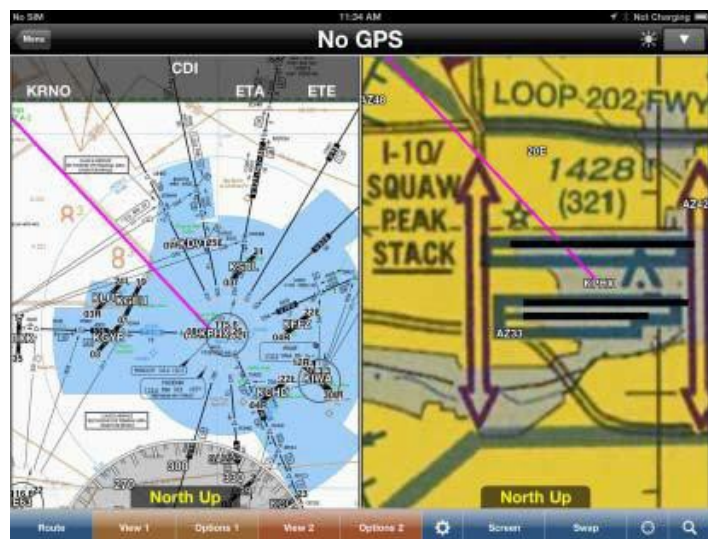
Figure 2. Example of digitized paper charts displayed on a tablet computer
