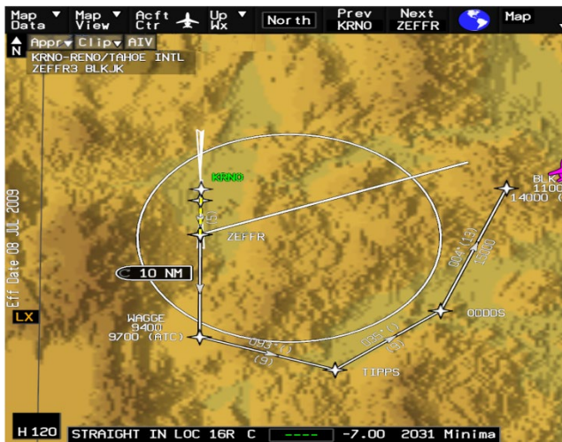
Figure 5. FMS flight plan supplemented by chart data
