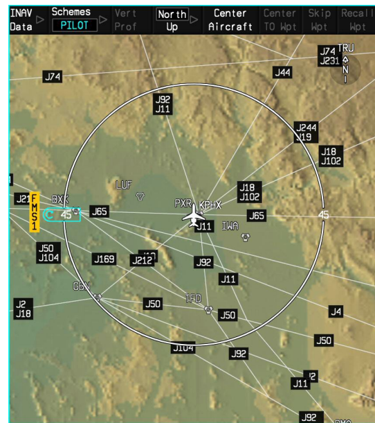
Figure 6. High/low airways on navigation display
