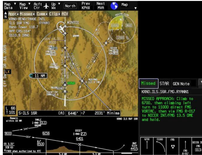
Figure 19. Shows IFR chart data integrated within a navigation display
