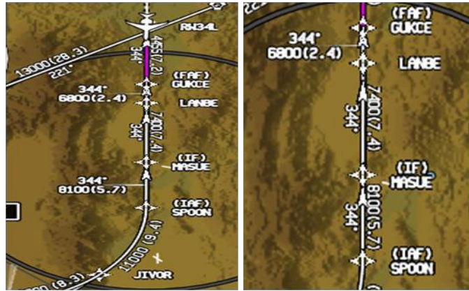
Figure 8. Benefits of an offset pointer drawn to the area where the data belongs
