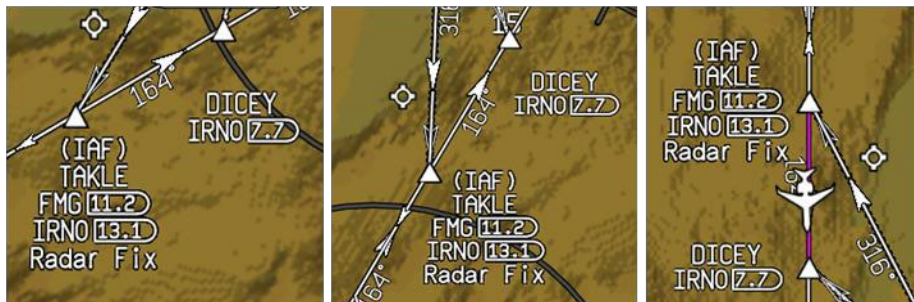
Figure C.3.1: As the track of the aircraft changes, text rotates to maintain proper reading orientation.
